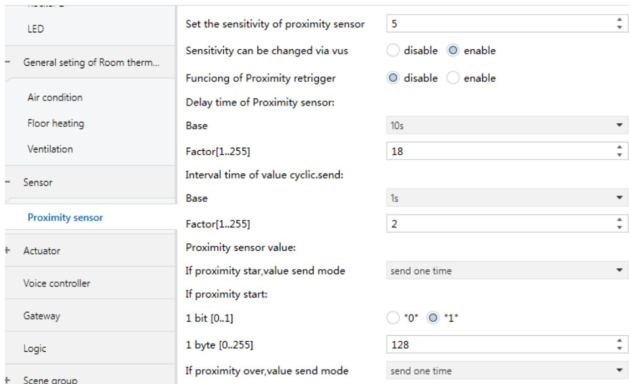
Figure 3.4.1 Parameter window“Proximity sensor”
