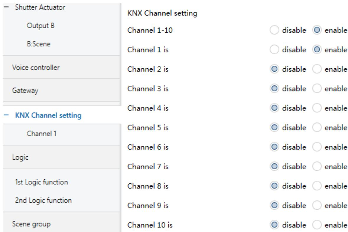
Figure 3.8.2 Parameter window “KNX Channel setting”
