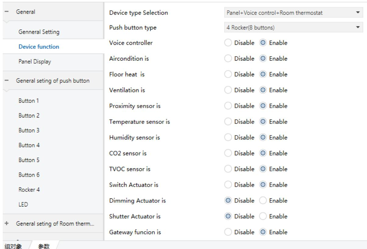
Figure 3.1.2 Parameter window “Device function”
