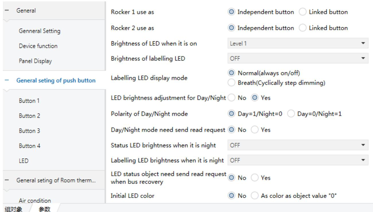
Figure 3.2.1 Parameter window“General setting of push button”
