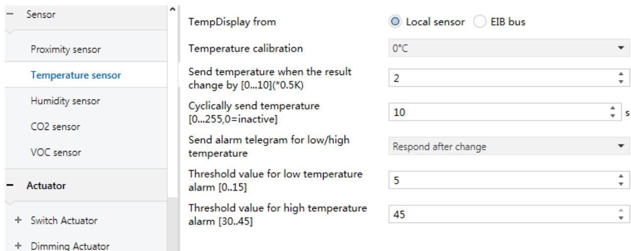
Figure 3.5.1 Parameter window “Temperature sensor sensor”
