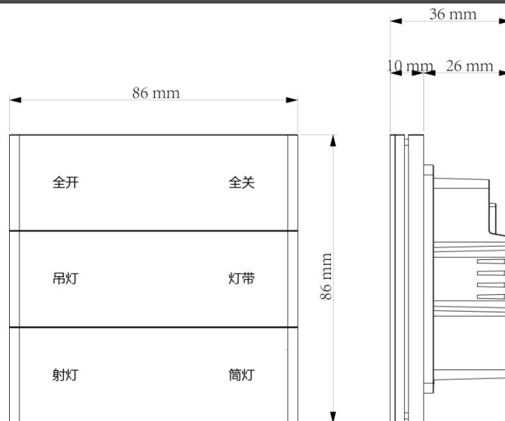
Figure 2.2.3 Structural dimension diagram of three pairs of associated key panels
