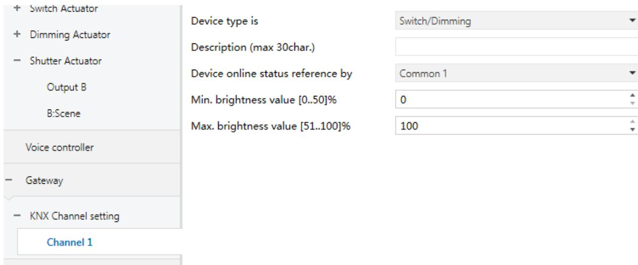
Figure 3.8.4 "Channel X - Switch/Dimming" parameter Settings page
