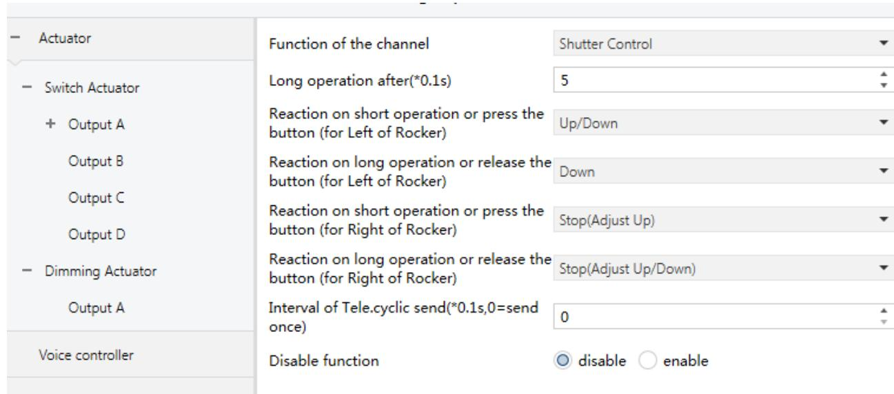
Figure 3.2.14 Parameter window“Rocker X- Shutter control”
