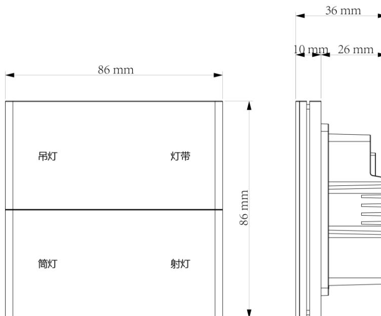
Figure 2.2.2 Structural dimension diagram of two pairs of associated key panels
