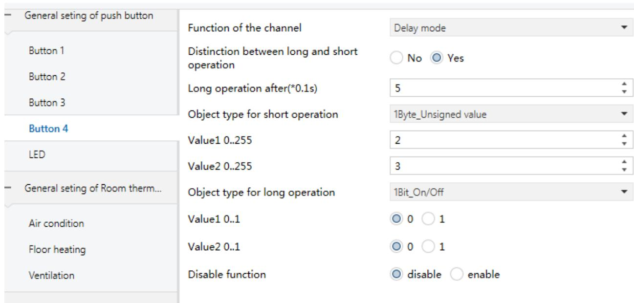
Figure 3.2.10 Parameter window“Button X- Delay mode”
