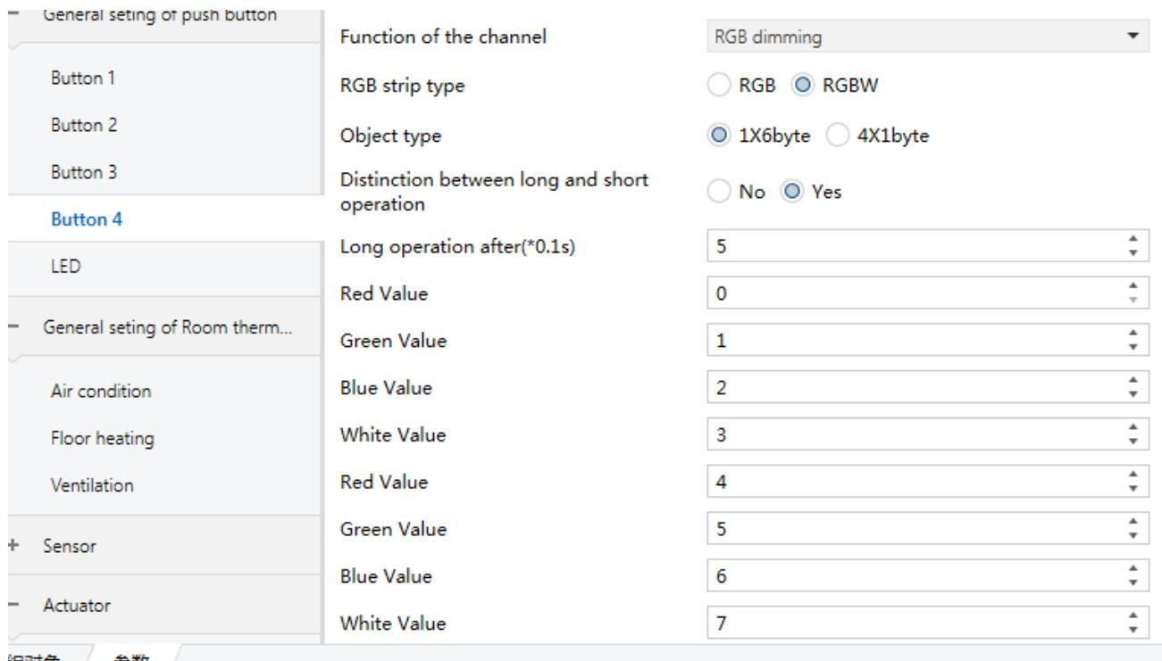
Figure 3.2.8 Parameter window“Button X- RGBW dimming”-2
