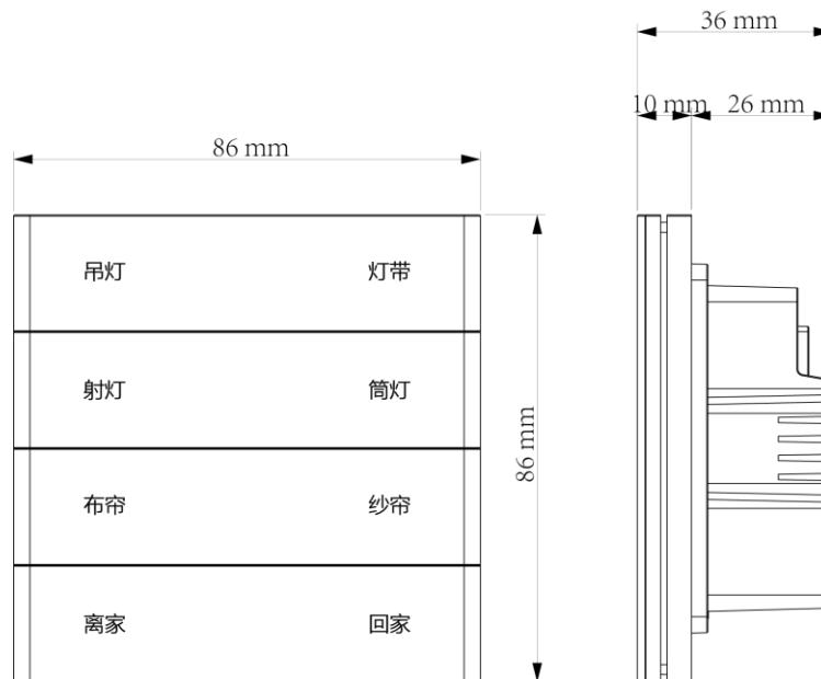
Figure 2.2.4 Structural dimension diagram of four pairs of associated key panels
