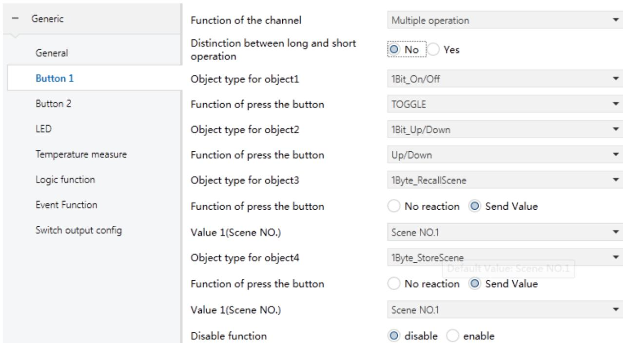
Figure 3.2.9 Parameter window“Button X- Multiple operation”
