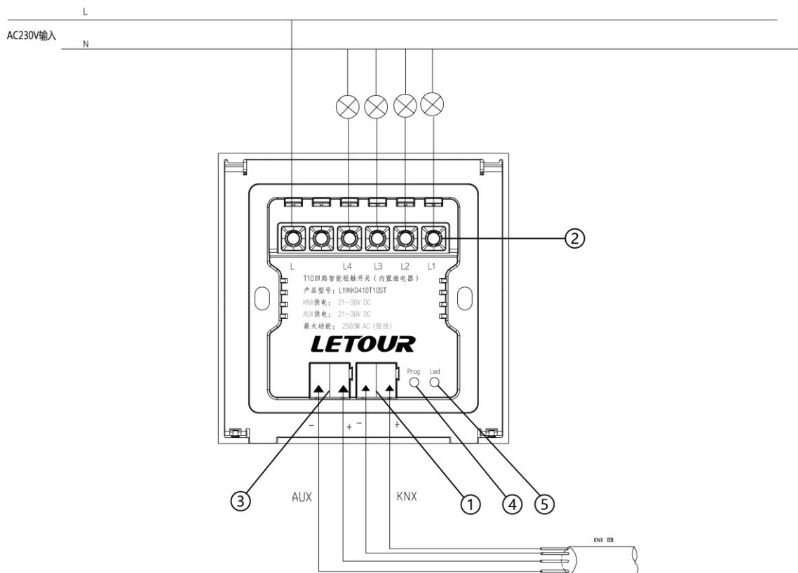
Figure 2.3 T10 Intelligent switch panel wiring diagram
