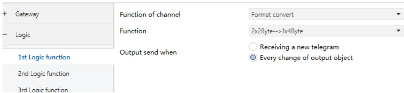
Figure 3.9.4 "Logic Format Convert" data conversion parameter Settings page
