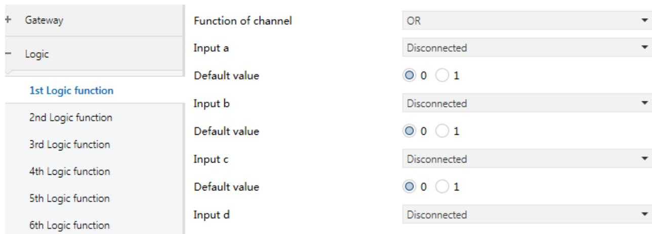
Figure 3.9.2 parameter window "Logical operations AND/OR/NAND/NOR/XOR"
