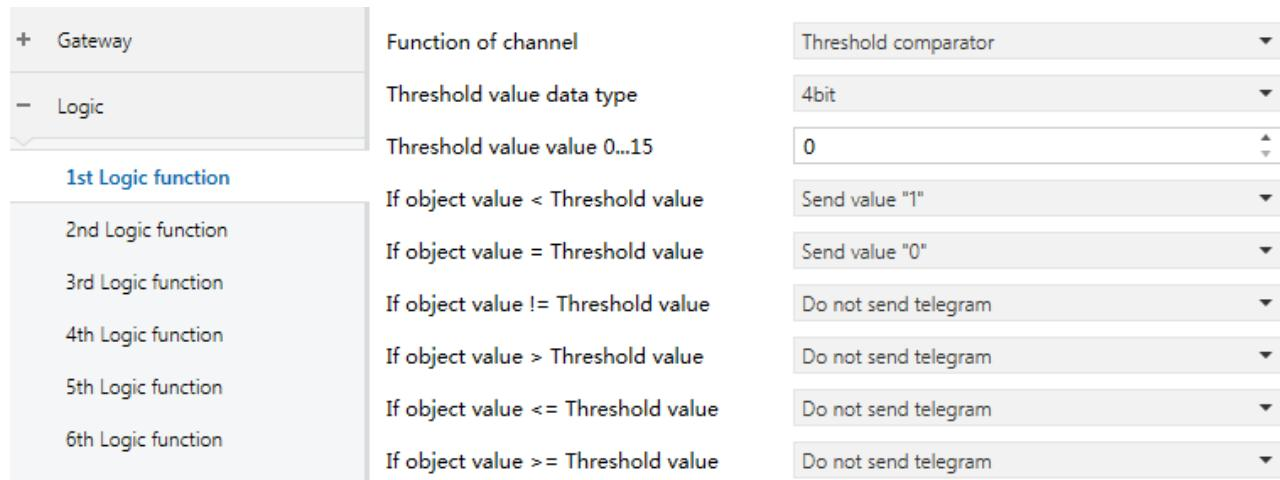
Figure 3.9.3 parameter window "Logic Threshold comparator"
