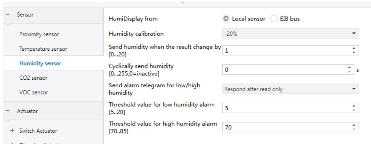
Figure 3.6.1 Parameter window “Humidity sensor”
