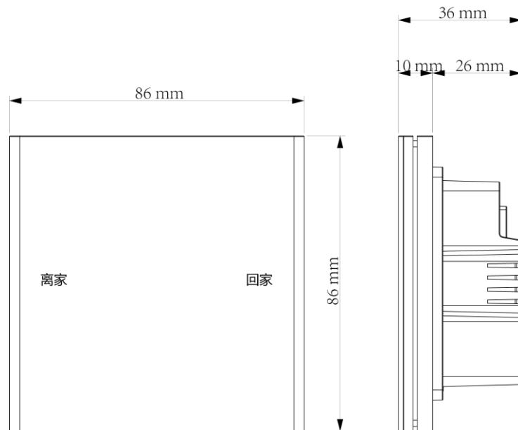
Figure 2.2.1 Structural dimension diagram of a pair of associated key panels
