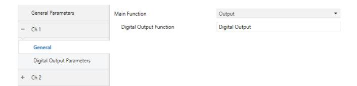
With this option, the channel is used to light the LED lamps or trigger the logic gates. The LED lamp can be connected directly (No need for a series resistor).
