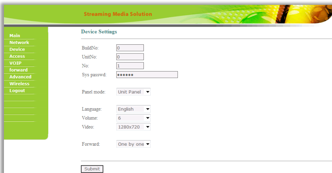
Figure 25: Device Settings Interface of the Outdoor Intercom
