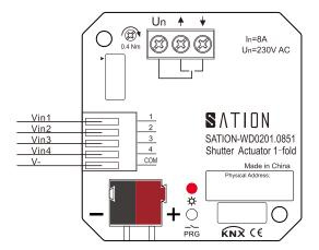
Note: High level is input 3.3V~24VDC
