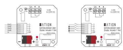
Note: low level includes the positive signal of the OC gate input and input level below 1VDC
