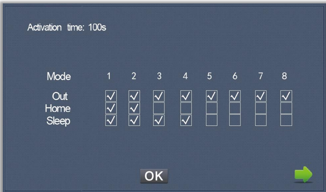
Fig. 23 : Scene interface of the Indoor Panel
