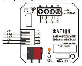
Note: High level is input 3.3V~24VDC
