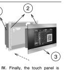
placed in the mounting box by moving in the direction of the dashed arrow. Then it is screwed to the mounting frame through the screw slots on the 4 corners of the panel. Magnetic materialled lath with 2 horizontal holes on it should be attached to the lower part of the panel and the other one is attached to the upper part of the panel and the mounting process is completed.
