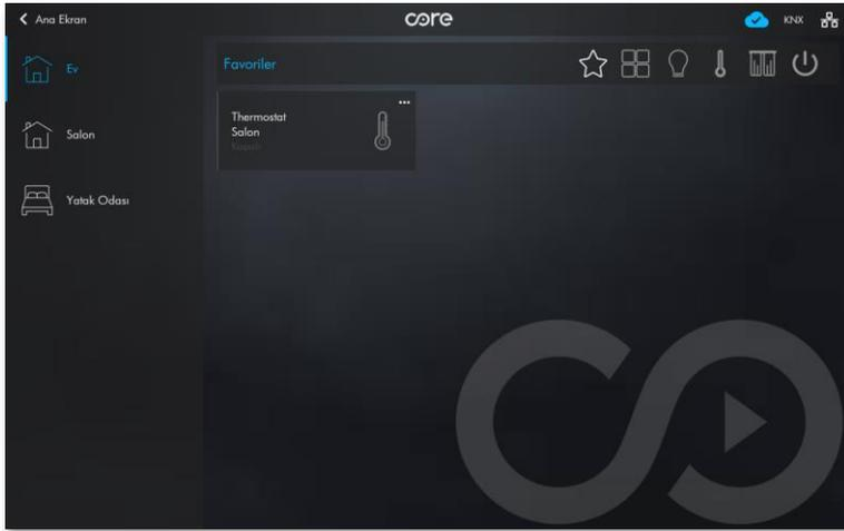
In summary view, operation mode and room temperature of thermostat is monitored. Just tap device to reach detailed view.
