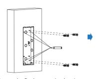
Insert the flush-mounting box in to the hole and mark the the positions of the four holes of the flush-mounting box on the wall, then take off the box and drill the holes on the marked positions using 5 mm drill bit hand drill before inserting the plastic anchors in to the drilled holes.
