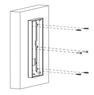
Place the wall-mounting box closely against the wall while lining up its four holes with their corresponding drilled holes and then fix the wall-mounting box on the wall by tightening four ST x 20 screws and two M4x30 screws to the plastic wall anchors.
