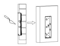
Make sure that the flush-mounting box are well tightened and its upper and lower folded edges are fit snugly against the wall, fill in the gap between the wall and the flush-mounting box using cement or non-corrosive structural adhesive and wait until the cement is hardened before proceeding to the next step.
