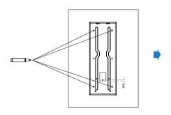
According to the position of the wire on the wall, put the wall-mounting box closely on to the wall and mark the four positioning holes, while making sure that relative positions between wall-mounting box and wiring hole are correct.
