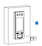
Press the card reader touch plate in to the card reader opening.
