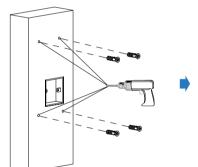
Take off the box and drill the four marked holes using 5 mm drill bit hand drill before inserting the plastic wall anchors into the drilled holes.
