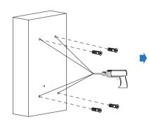
Drill the marked holes using 5 mm drill bit hand drill before inserting plastic wall anchors in to the drilled holes.
