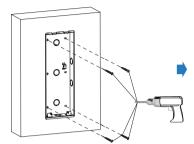
Break off the round knock-out wiring holes and lead the wires through the corresponding hole in to the flush-mounting box, then press the flush-mounting box in to the square hole. The upper and lower folded edges of the flush-mounting box must fit snugly against the wall. Then fix the box using the four plastic wall anchors and the four ST4x20 screws.
