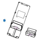
Choose a suitable size rubber plug (small, large and medium) to hold down the wires, while tearing off the adhesive sticker on the selected rubber plug and stick it on to the X915 back cover and then tear off the adhesive sticker on the other rubber plug of the same size and stick it on to the back cover in the position as indicated in the drawing.
