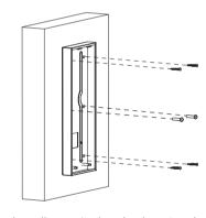
Place the wall mounting box closely against the wall while lining up its four holes with their corresponding drilled holes and then fix the wall mounting box on the wall by tightening the four ST4 x 20 screws and two M4x30 screws to the plastic wall anchors.
