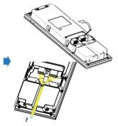
Connect the wires to the terminal blocks as needed (for details, refer to "Device Wiring"), then insert the terminal blocks into the corresponding interface of the main board as indicated in the drawing according to the number of PIN.
