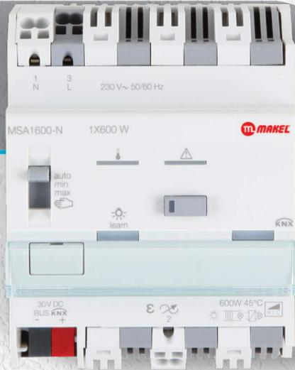
The KNX with single channel dimmer devices can be used to dim halogen, 220V led, fluorescent, incandescent and cfl lamps using the smart system. The device is capable of providing drive for lamps 600 watts 1 channel. These products are with automatic load detection and manual adjusting, to control the compact fluorescent 220V LED lamps more efficiently.
