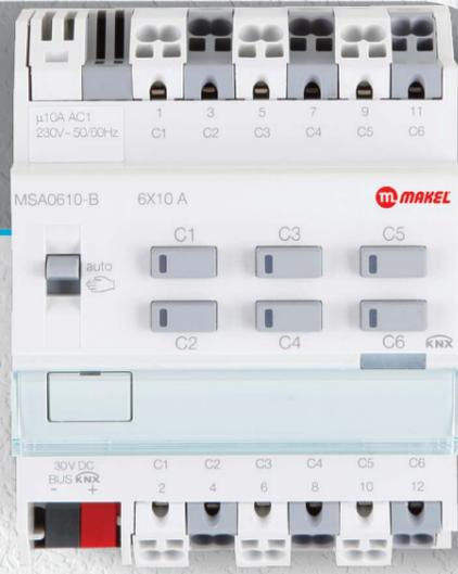
You supply energy to or cut the energy off from the control module connected KNX on/off. With a current capacity of up to 10A, number of outlets that can be increased to 6 channels and manual and automatic use functions, they are essential components of smart building systems.
