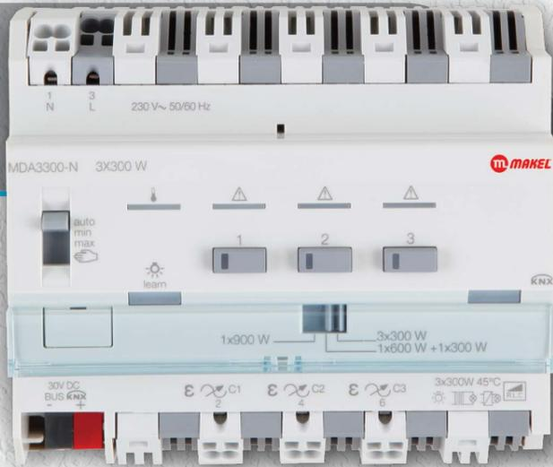
The KNX with 3 channels dimmer devices can be used to dim halogen, 220V led, fluorescent, incandescent and cfl lamps using the smart system. With a total capacity that reaches 900 Watts, lamps can be maintained at 300 Watts for each of three channels, 300W and 600W for two channels and 900W for a single channel.
