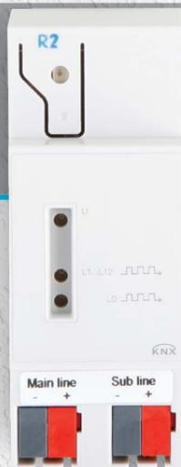
Line coupler devices are one of the basic elements of the KNX system. By using these devices lines to which up to 63 devices can be connected on each KNX connection can be created. Line coupler can create smart home systems comprised of up to 65,000 devices in total. Line coupler devices can also be used as repeaters on the same line when necessary. Line coupler devices filter traffic and prevent messages from going to unnecessary lines.
