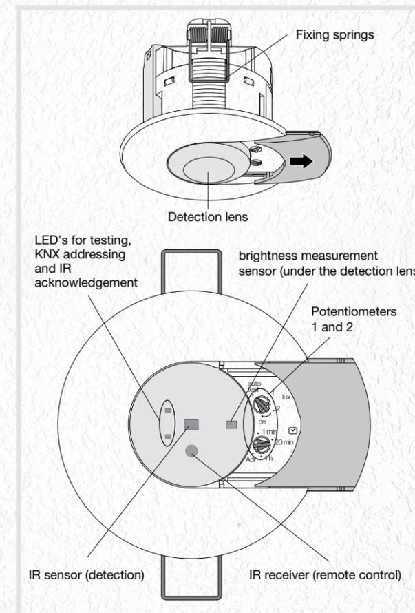
Occupancy sensors MRP 1000 are presence detector designed to detect low amplitude movements (movements from body or arms). Detection is by means of the pyroelectric IR sensor under detection lens. The occupancy sensor measures the brightness in the room on continuous basis and compares it to the level present on the potentiometer by ETS.
