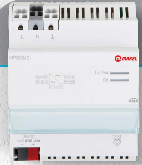
The power supply MPS0640 generated the system voltage, which for the operation of the smart home devices. The system voltage generated by the MPS0640 meets the requirements of the protection measures SELV (safety extra-low voltage).
