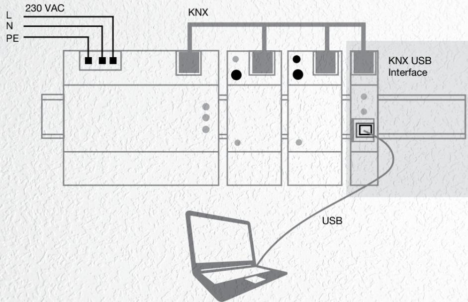
This interface is for establish a bidirectional connection between a PC and the KNX installation bus. The USB connector has a galvanic separation from the KNX bus. Both ETS (Engineering Tool Software) versions ETS3 or later and some visualization tools support this interface.
