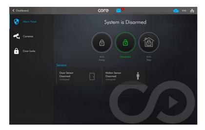
KNX Sensor Accessory type is displayed in security menu of user interface. The sensor's name, icon, arming status and trigger status are displayed.
