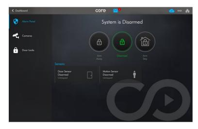
Modbus Sensor Accessory type is displayed in security menu of user interface. The sensor's name, icon, arming status and trigger status are displayed.
