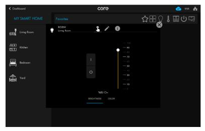
You can find detailed view of RGBW Dimmer Accessory in the left hand side. Central on/off and central brightness control and status information and changing brightness value in form of drag and drop are displayed and controlled under this function
