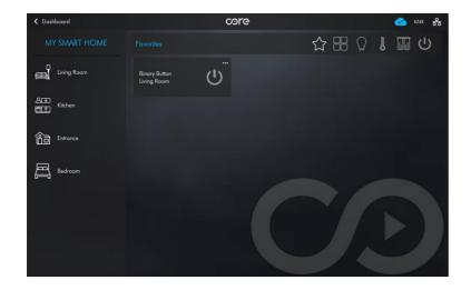
In summary view, name and icon of the device is displayed. Only monitor acknowledge when data is sent, because there is not any status related to this accessory. Just tap device to reach detailed view.
