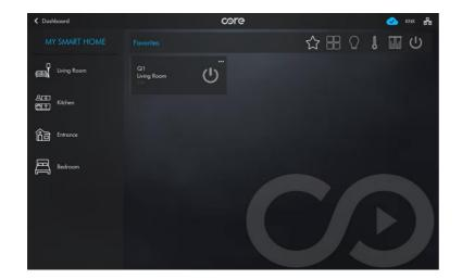
System I/O Switch Accesspry type is displayed in the user interface in the category determined by the integrator. The name, icon and status of load are displayed.
