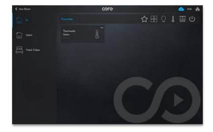
In summary view, operation mode and room temperature of thermostat is monitored. Just tap device to reach detailed view.
