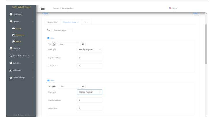
Data Type: Modbus thermostat operation mode address type
