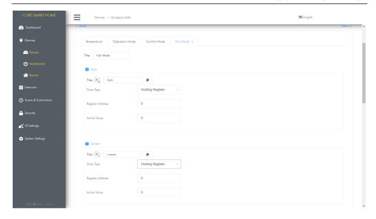
Data Type: Modbus thermostat fan speed address type
