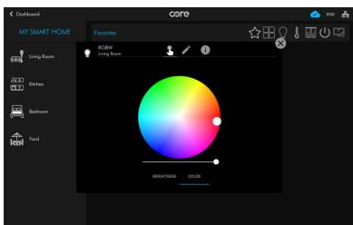
You can find detailed view of RGBW Dimmer Color function group in the left hand side. The Color Wheel and White light brightness value, are displayed and controlled under this function
