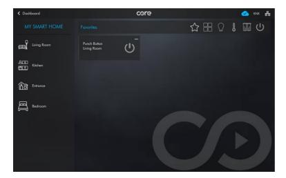
In summary view, name and icon of the device is displayed. Only monitor acknowledge when data is sent, because there is not any status related to this accessory. Just tap device to send value. Tap 3 dots in the upper right corner to reach detailed view.
