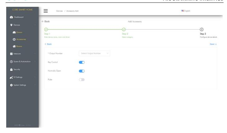
Output Number: Number indicating which output of Siemens Logo the switch is connected to
