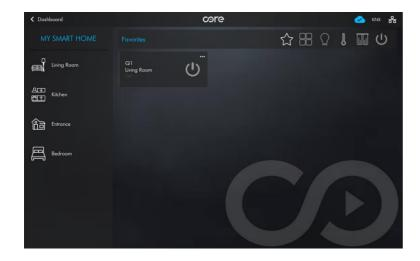
Modbus Switch Accesspry type is displayed in the user interface in the category determined by the integrator. The name, icon and status of load are displayed.
