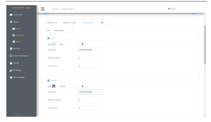
Data Type: Modbus thermostat control mode address type
