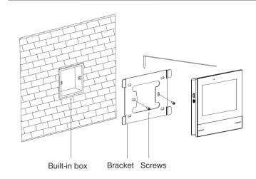
The following figure, shows a proper location of the installation:
